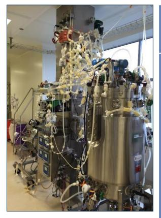
CPC Connectors on Bioreactor Fluid Transfer Manifolds Tech Overview
