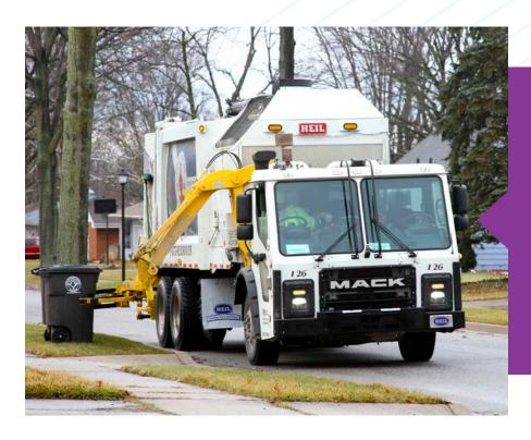
The Heil MultiPack® takes functionality to the next level by providing fleet owners with the industry's only garbage truck that combines a rearloading hopper with a highly productive Python® automated arm. With the MultiPack, an operator can throw bulk waste into the rear hopper – while operating the arm to continue with automated collection.
